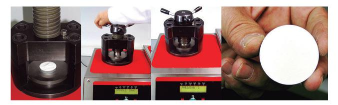
The technique consists in compressing the particles of the dust sample (by themselves or with a binder) until getting a perfectly homogeneous disk with a flat surface, mechanically robust and without cracks or dust.
