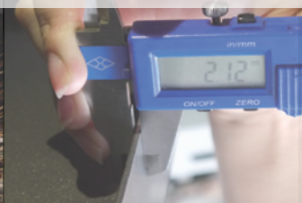
Thickness of 316L stainless steel >2mm
