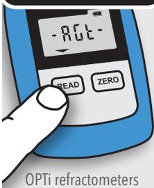
OPTi refractometers have an "AG Test Mode" that uniquely facilitates verification using long-life NIST traceable AG Fluids without the need to consider the scale or ATC type.
