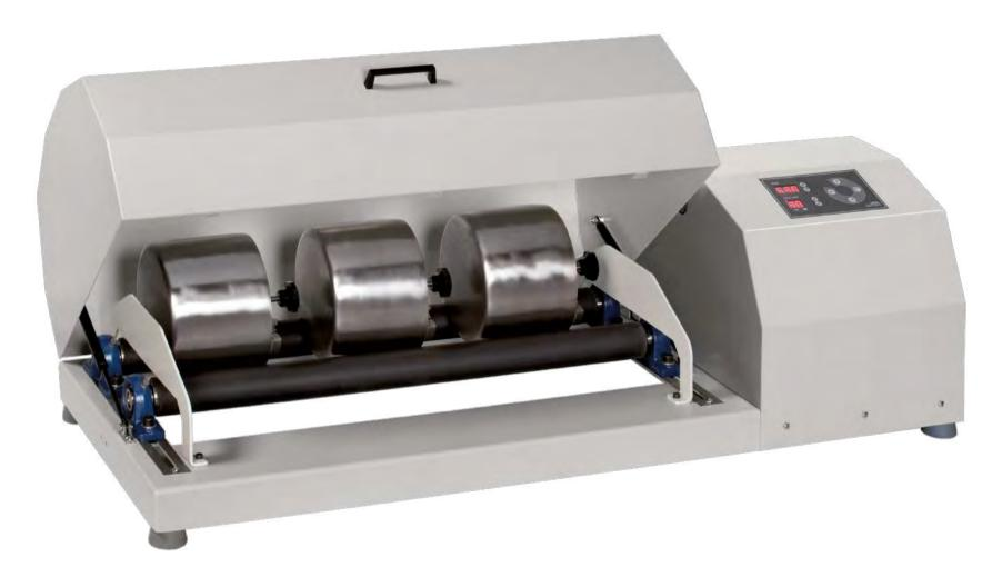
The ball mill splits the sample by using repeated hits against the balls. It moves along an arc of a semicircle due to the dragging of the pitcher in the cylinder motor. Isolated jars prevent the contamination of samples.
