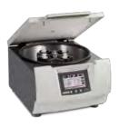
Max. Capacity 4 x 60 ml Max. Speed 1.801 xg / 3.000 RPM Screen Type
